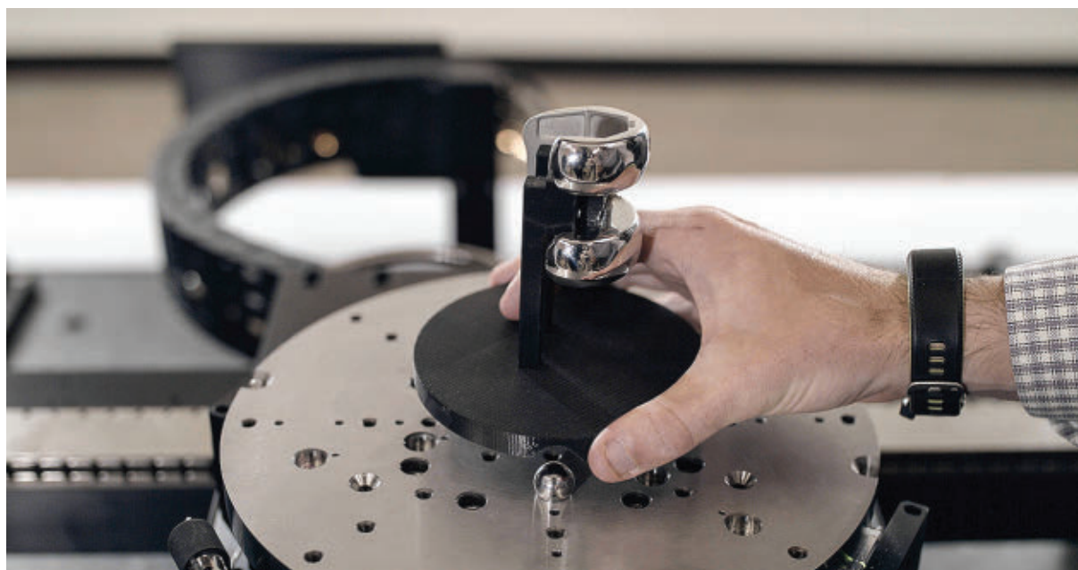
Further time is saved by the simplicity with which parts and assemblies can be placed on the measuring table, instead of requiring complex positioning fixtures. The variety of available sensors allows 3D measurement or any kind of surfaces including mirror-like ones.
